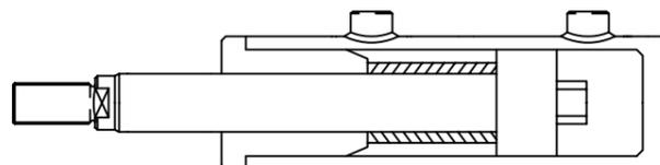
THE PISTON ROD IN A CYLINDER ACTS AS A COLUMN UNDER THRUST (PUSH) CONDITIONS. IT IS, THEREFORE, SUBJECTED TO BOTH COMPRESSIVE STRESSES AND BUCKLING STRESSES. CONSEQUENTLY, IT MAY BE NECESSARY TO INCREASE THE ROD DIAMETER TO ACHIEVE THE NECESSARY COLUMN "STRENGTH".
